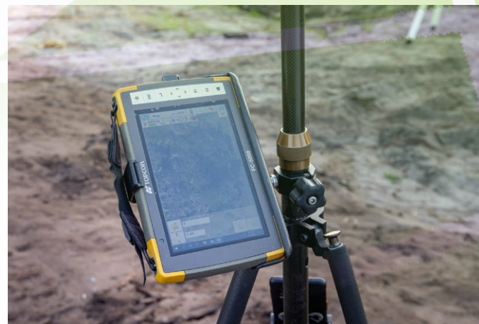
Atlantic's teams use Topcon FC-5000 field computers for on site data entry and transfer. Cesiro says the unit—which features front- and rear-mounted cameras—has made that facet of the job fast and easy.
