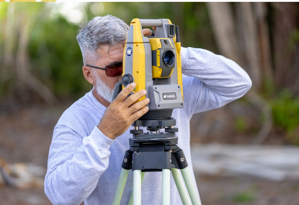
The flexibility of the GT-503 to switch from robotic prism to prismless allows Cesiro to jump behind the instrument and collect data in a more conventional manner. Being able to switch from GPS to robotic to prismless means obstacles are no longer a concern.
