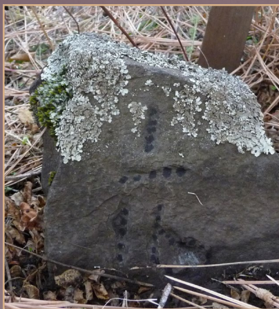
1909 Co. Surveyor's W1/16th Stone. Notice the rounding effect of electrolysis.
