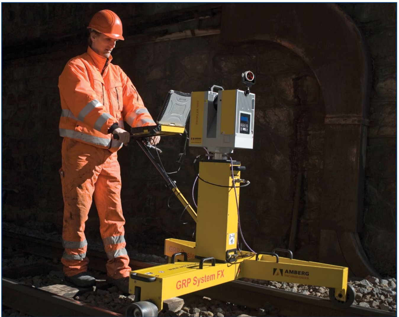
Top of the line GRP 5000 trolley with the Profiler 5003 3D scanner.
