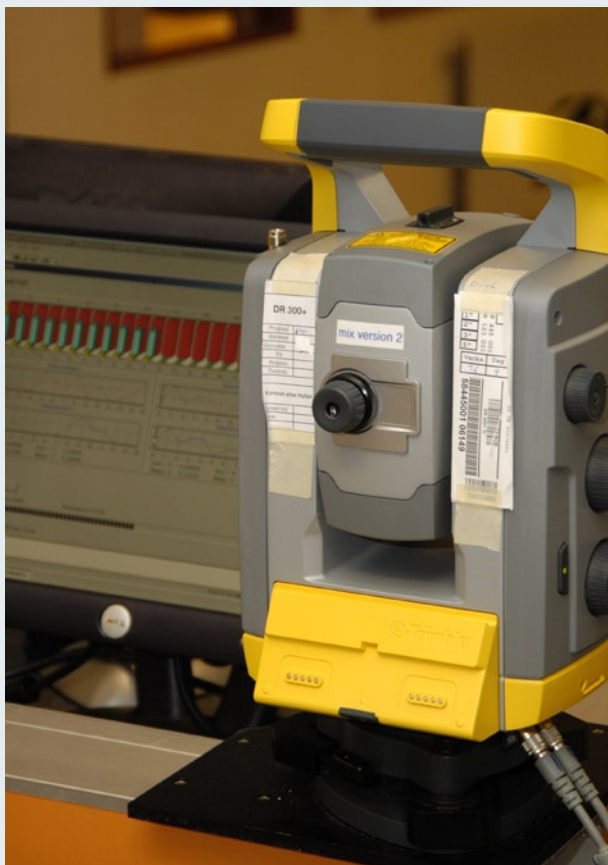
Trimble S6 total station. Note bar code that is part of the factory's automated tracking.
