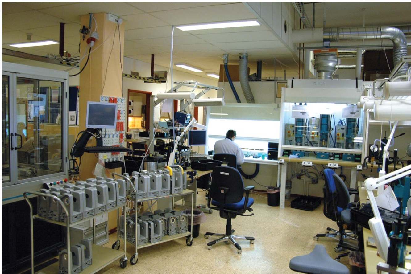
One of many pre-check stations before components are moved into the final S6 production line. For the 5600 series of instrument, one person performs all the steps in the assembly. For the new-gen instruments such as the S6, production takes place on a line, with each person in the line performing one or more steps.
