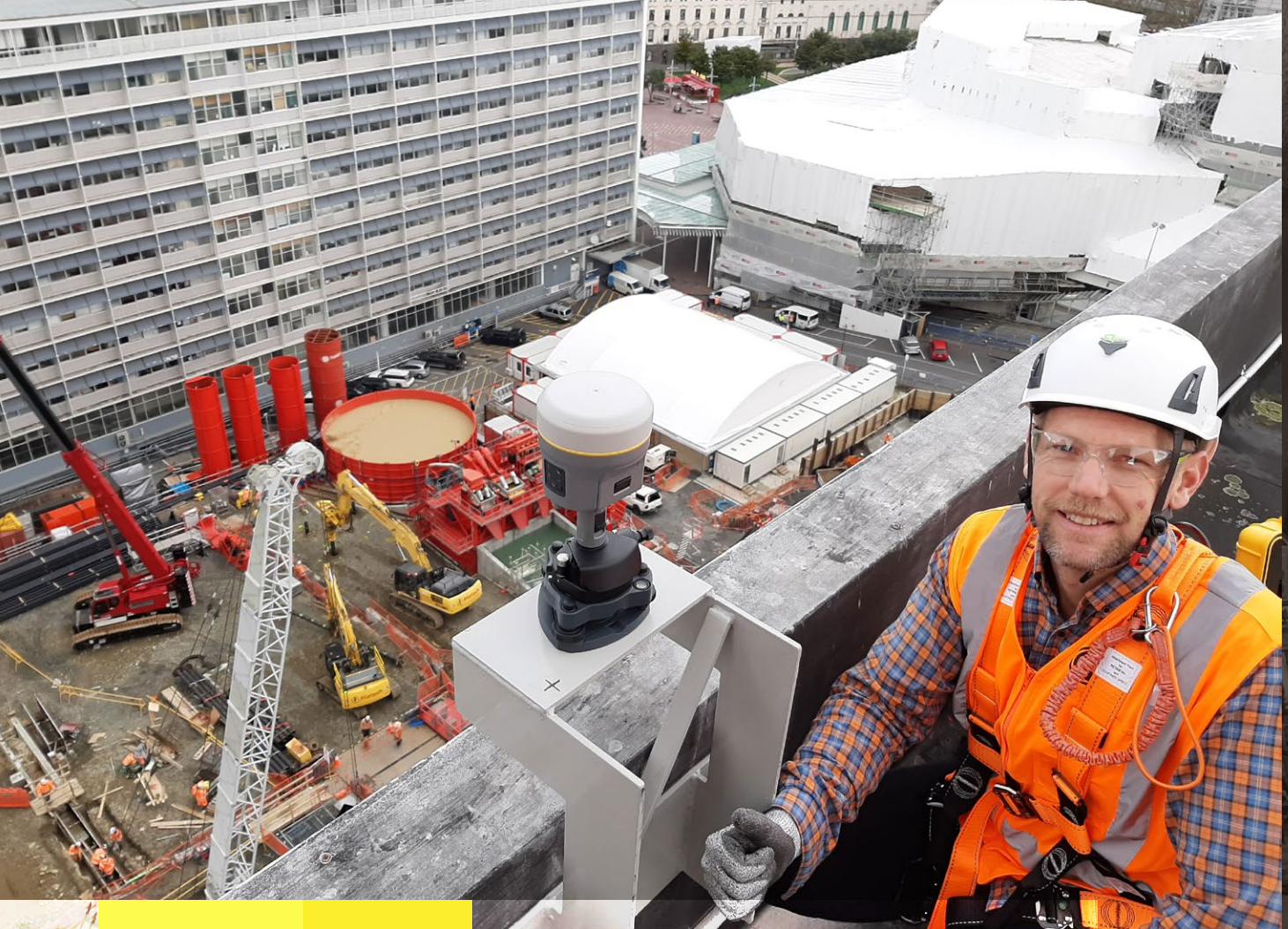
A Trimble R10 GNSS receiver acquires static observations above the Aotea station work site.
