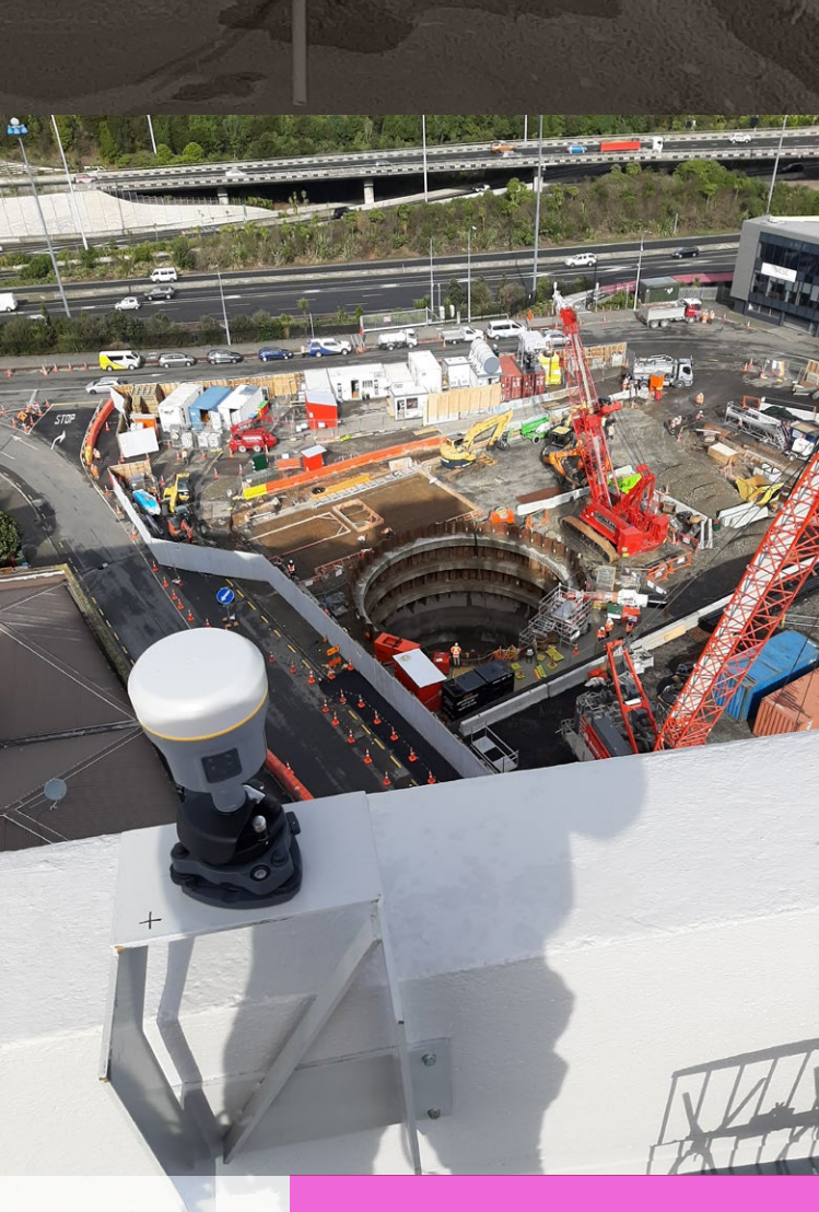
A Trimble R10 GNSS receiver acquires static observations above the Karangahape station work site.
