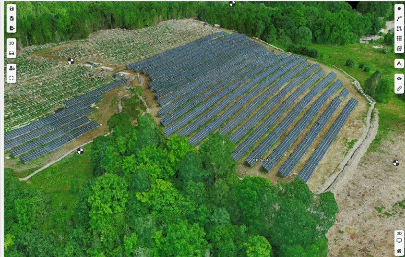
Carlson PhotoCapture perspective view of partially completed solar farm. The black and white targets are the ground control points.
