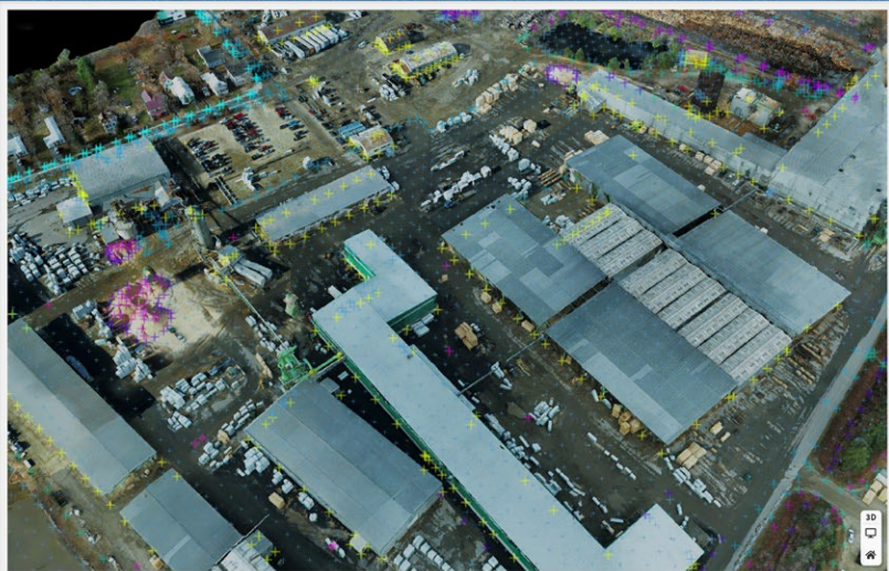
Digitized elevation breaklines for a lumber mill site.
