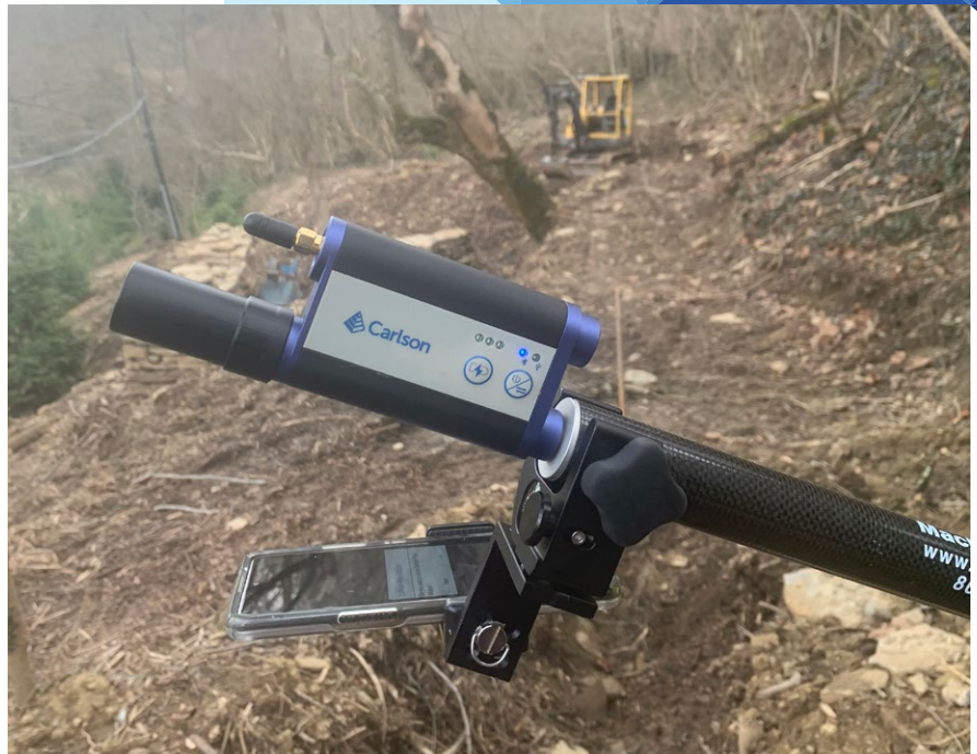
The Carlson xML2 system consists of any Android phone with photo capability mounted as shown, along with the top-mounted xML with built-in GNSS. Carlson Layout on Android provides the RTK engine. No cables or wires are involved.
