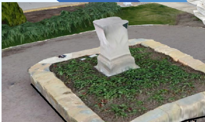
Pedestal for Daniel Boone, mapped in 3D by PhotoCapture. Pick on map using Polyline option at right, then draw to CAD. Note "Bare Earth" feature, where tree branches are flattened to ground level.
