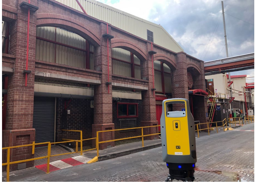
Roelvert uses the Trimble X7 to capture as-is information for upgrades at the Chamdor Brewery in Krugersdorp, South Africa.
