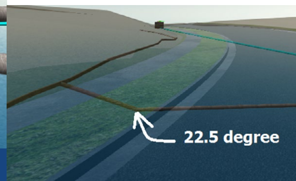
Regulations even govern pipe deflection angles between pipe segments, and allowable fittings
