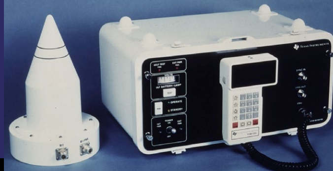
A Texas Instruments 4100, or TI 4100, which was used in early GPS surveying experiments. SOURCE: NOAA
