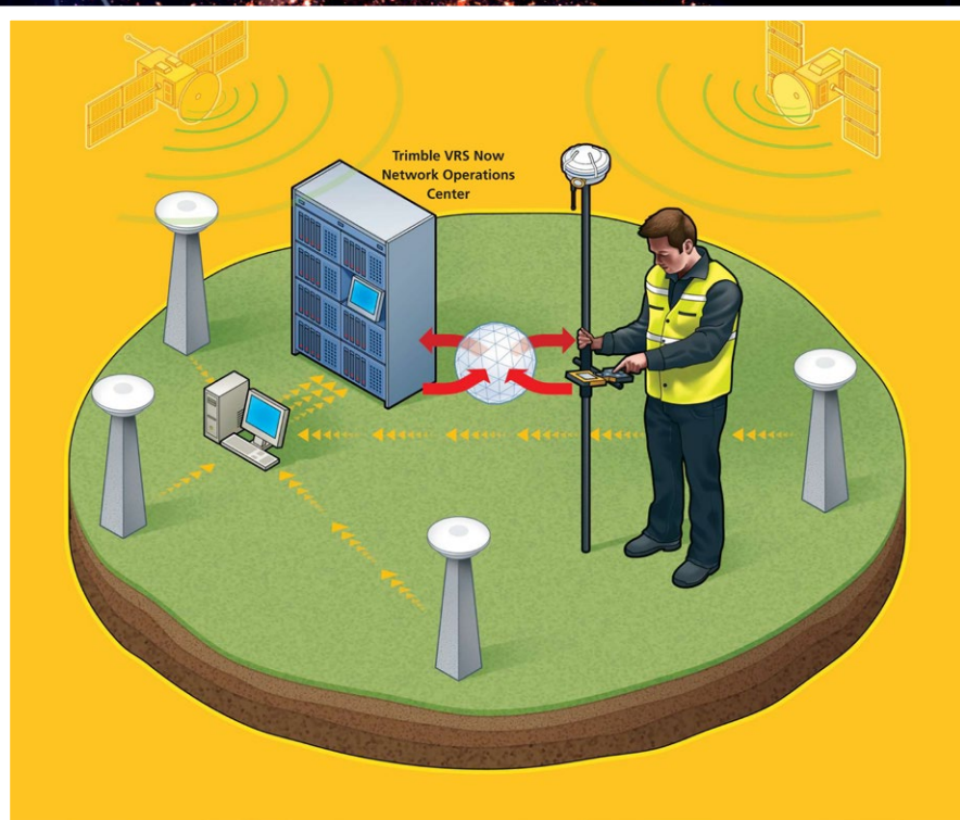
Illustration of RTN/VRS technology, a precursor to Trimble RTX.
