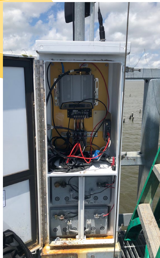
Part of the LSU C4G RTN network, this enclosure in the middle of Lake Borgne, La., holds two gel cell batteries, a solar charger, cell modem, cell booster and a Trimble Alloy GNSS reference receiver.
