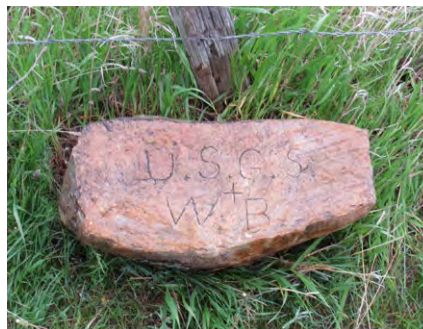
South Dakota licensed land surveyors Jon Collins and Linda Foster pose with the recovered "West Base" monument of the baseline that was established in 1891. The marked stone was found moved out of its original location and placed in a nearby fence.
