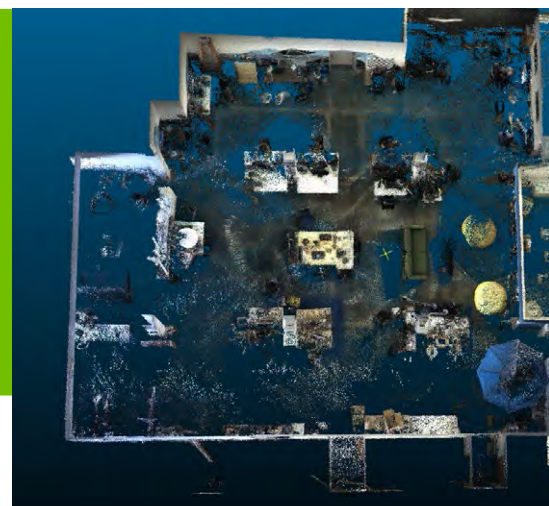
Floor-plan view of a PX-80 point cloud.
