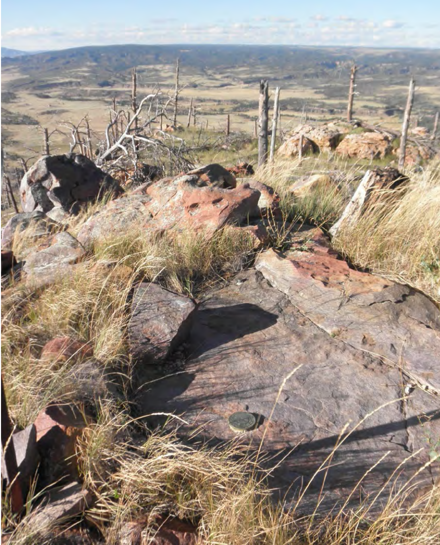
The copper bolt along the top edge of the flat rock was placed by USGS in 1897 and was designated station "Elk". In 1912, USC&GS occupied the same peak, but placed their own bronze disk just a few feet away and also designated their monument as station "Elk".
