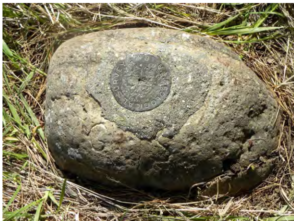
Triangulation station "Sammis" is one of the original monuments placed in 1893. The bronze disk was likely added during the reoccupation in 1897. The letters "G. S." can be seen along the bottom edge.
