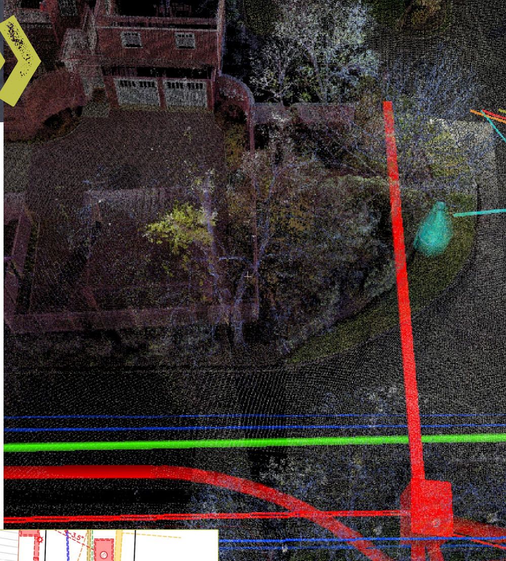
Subsurface utility mapping of underground environment on a university campus performed by DGT Associates.
