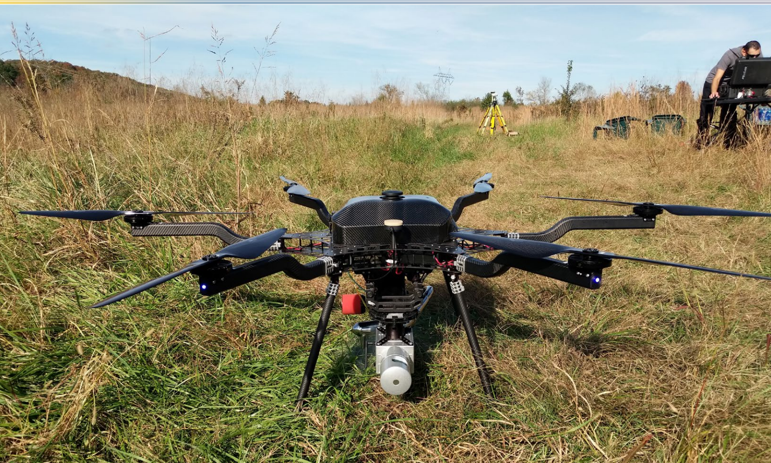
Harris H6 hybrid UAS equipped with LiDAR USA Snoopy A-Series HD sensor.
