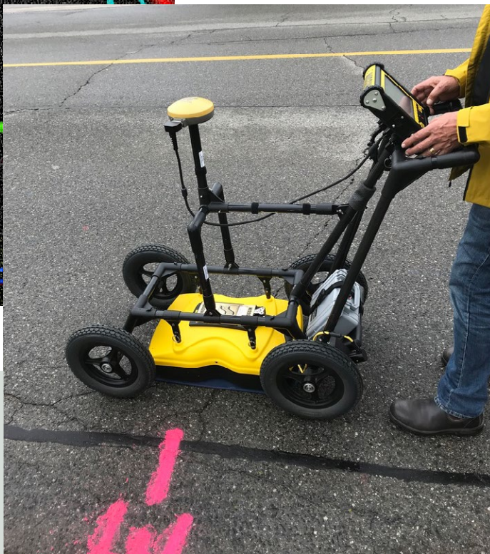
A DGT Associates crew member collects data of underground environment using a push-cart GPR system.
