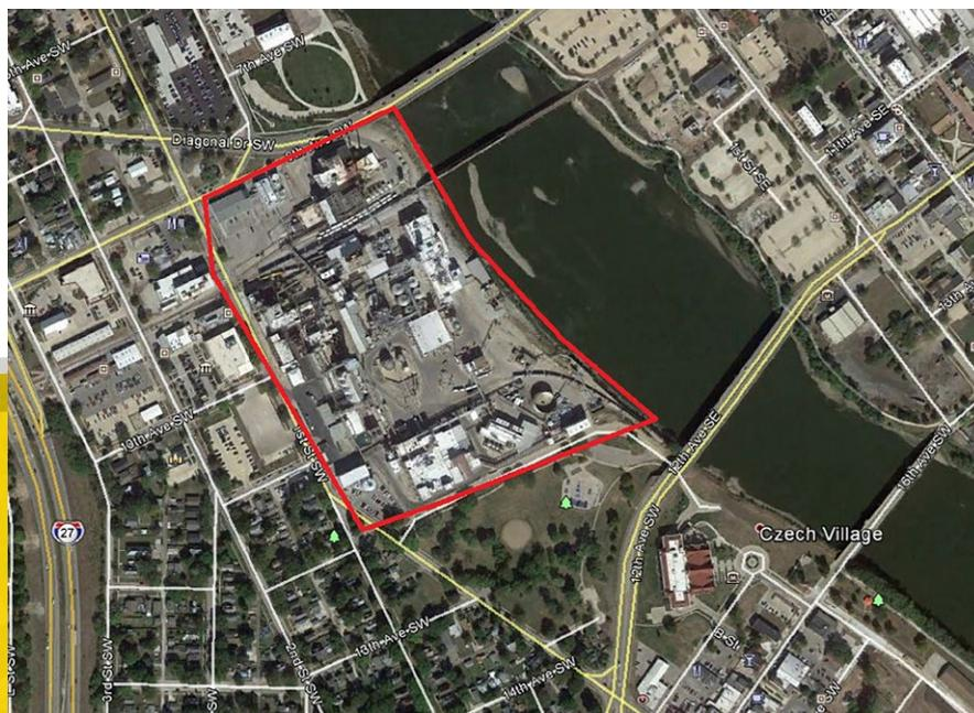
A section of the Site 2 as-built survey project. The area highlighted in red indicates a large industrial site that is inaccessible by foot because it’s lined by sheet piling walls. The long range of the SX10 enabled crews to capture that section from across the river.
