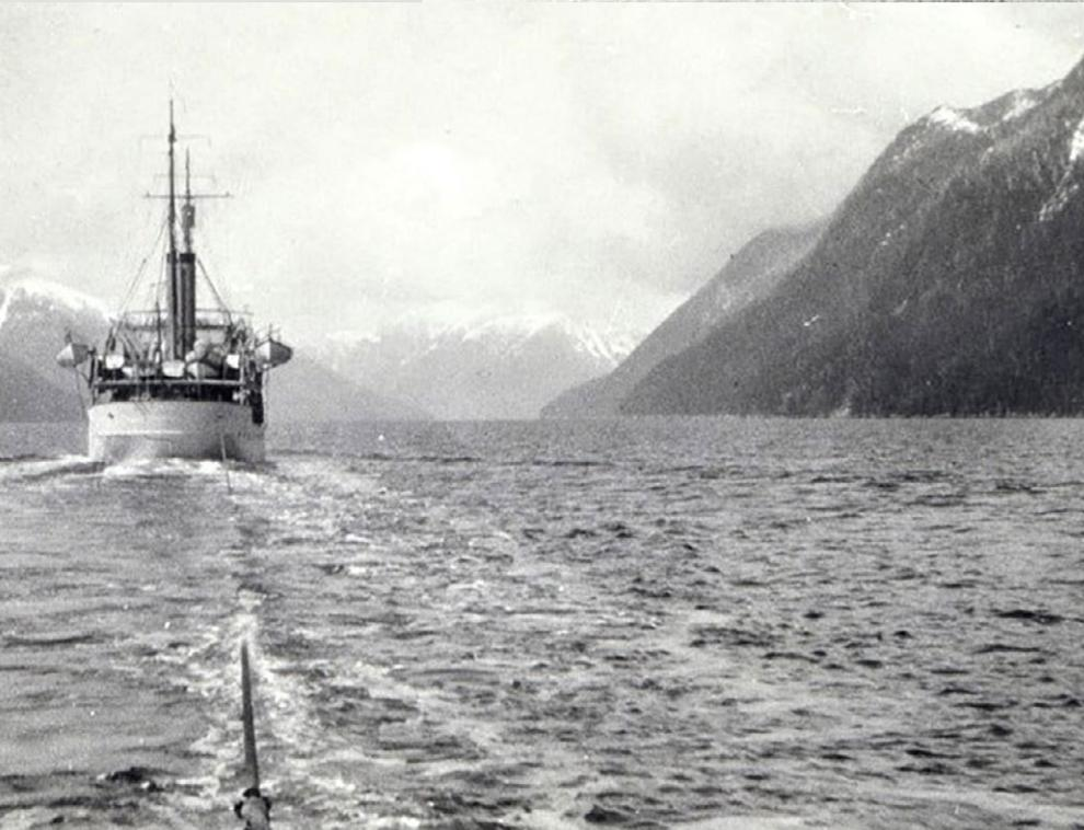
The stern of *Surveyor* as seen from the ship *Cosmos*. It is either being towed or possibly taking part in a wire drag operation to find submerged pinnacle rocks.
