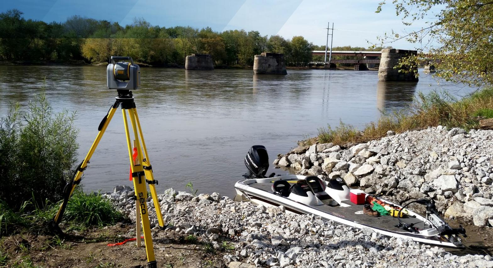
Because Site 1 was not accessible by foot, a crew had to navigate to control and scanning points by boat. Here the SX10 is set up to capture the railroad bridge in the distance and three old pier structures in the water.
