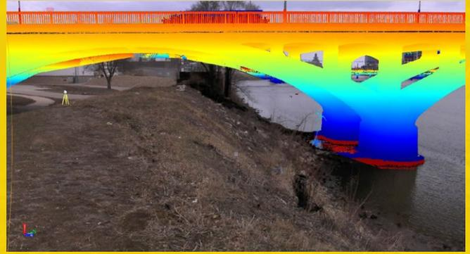
A shot of the 12th Ave Bridge from the SX10 internal camera with its equivalent point cloud view. This particular bridge had a 1.5-in clearance tolerance to the bottom of the bridge requiring a team to capture a 3D point every 0.125 to 0.25 inches.
