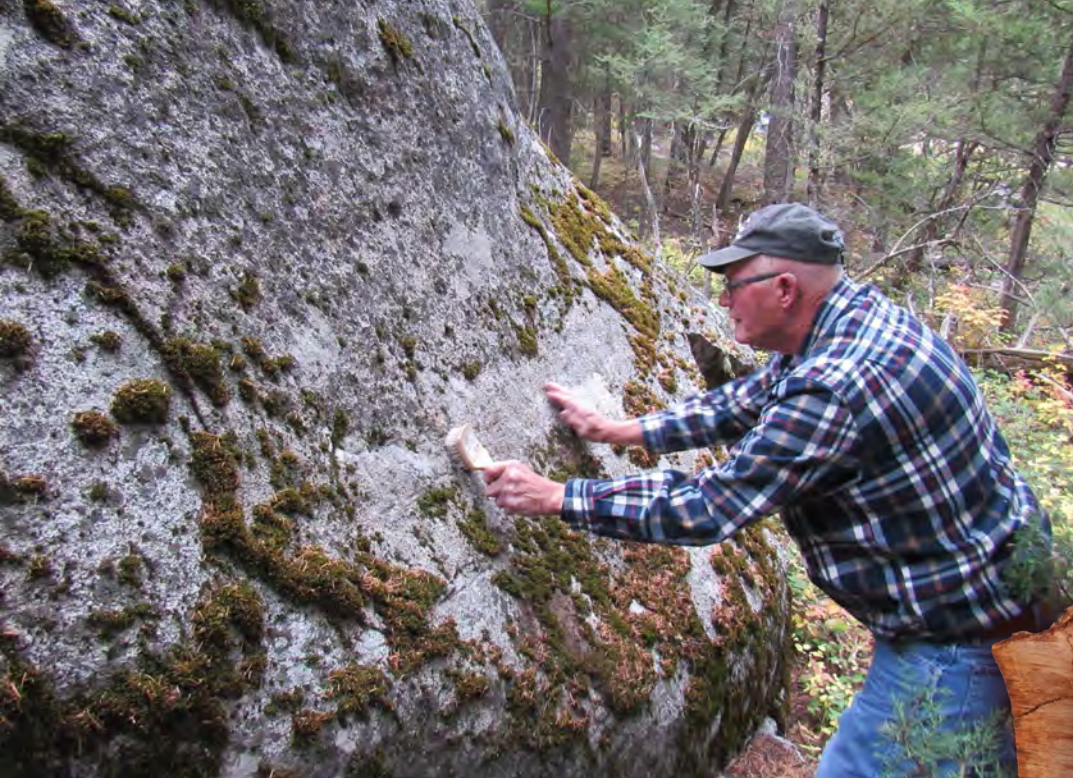
Gary Little of Montana, reveals the chiseled scribing on a large rock that reads "I. P. Boulder Mon. 1". This was Initial Point No. 1 in the Boulder Mining District of Montana when the "Princeton Lode" was surveyed in 1885.
