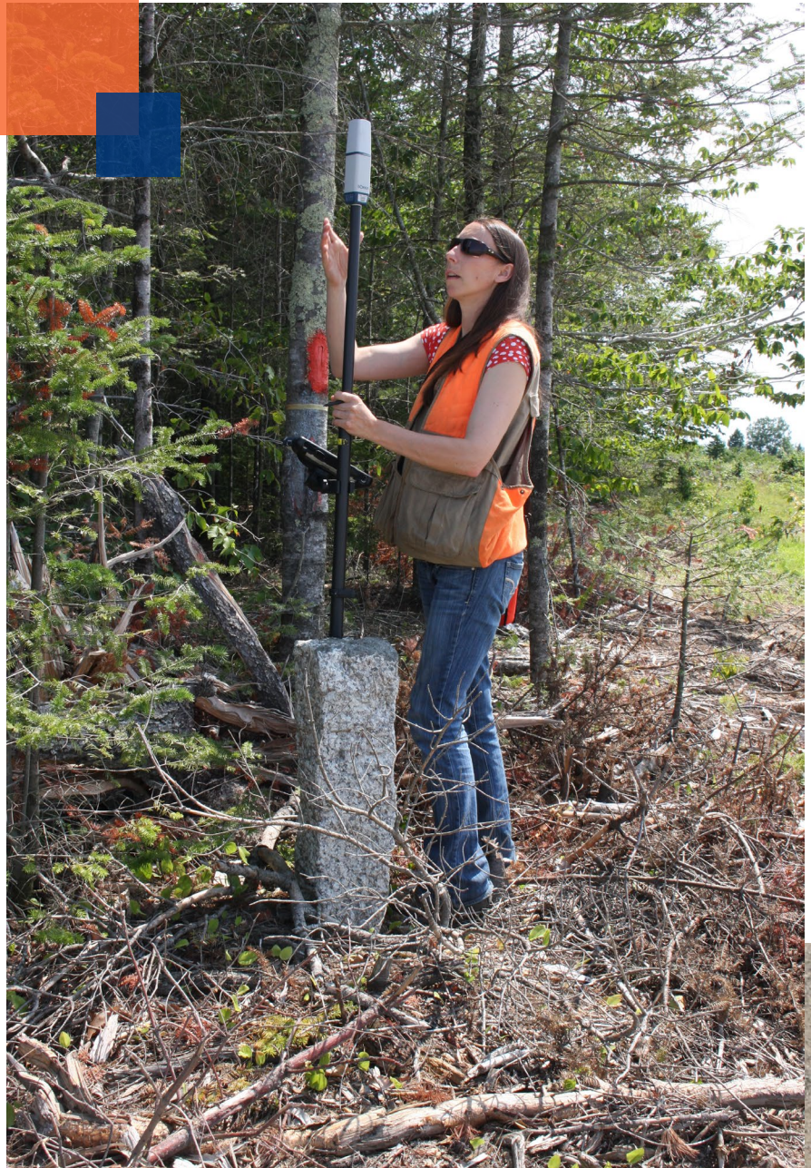
Using a Sokkia GCX3 paired with a Sokkia SHC5000 mobile tablet—also running Magnet 5 software—Hartson locates a granite post marking a property boundary corner. The receiver utilizes a cellular data connection to provide a virtual reference station, giving real time positioning without having to return to the office to process collected data.
