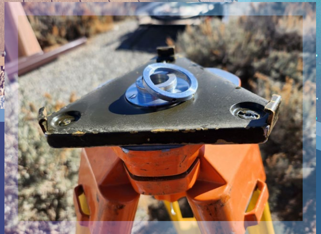
Tribrach busted too after tumbling off the deck into the gravel.
