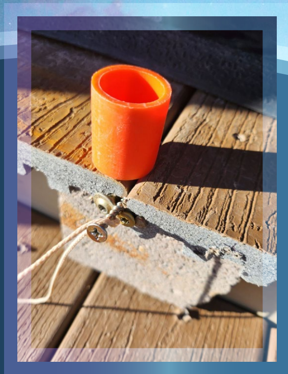
The two different screws set in the observatory deck for the azimuth of Polaris shots on five different nights either side of the one averaged to true north in the middle. The string line was used to align the telescope base plate.
