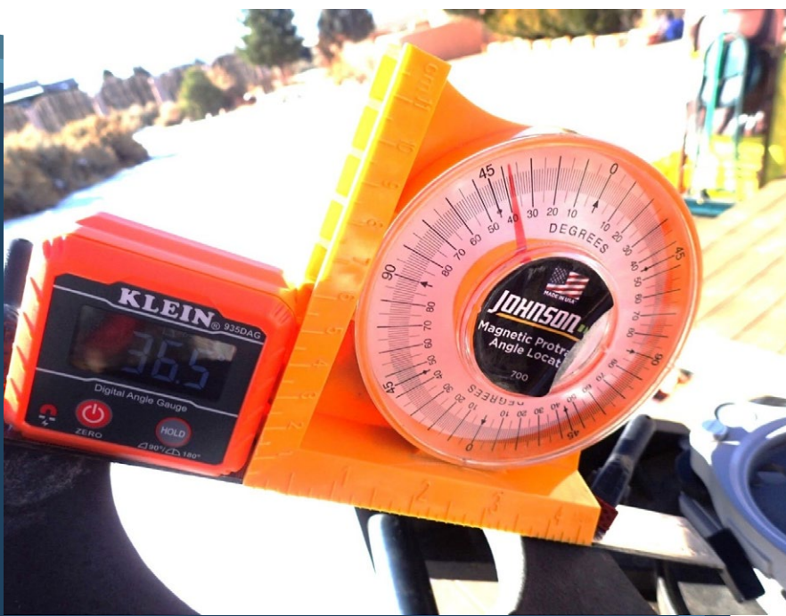
Digital and analog angle indicators on the telescope mount to set the latitude of the observing site near Taos, New Mexico.
